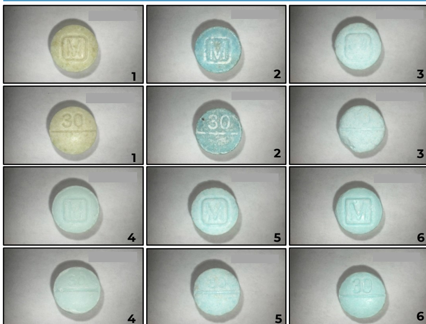
Figure 1. The tablets pictured were differentiated from each other based on differing colors and/or monogramming. The “30” marking on Exhibits 4 and 5 appear to be similar, but were differentiated based on color comparison and diagonal of M square measurement, which for Exhibit 4 was 4.95 mm and for Exhibit 5 was 5.85 mm. Exhibits 5 and 6 differed in the height of “0” measurement for the “30” monogram portion of the tablet. The height of zero measurement for Exhibit 5 was 1.50 mm and for Exhibit 6 was 2.21 mm. Exhibit 3 differed from the other exhibits because it appeared degraded and the monogramming could not be visually compared to the rest of the exhibits.
